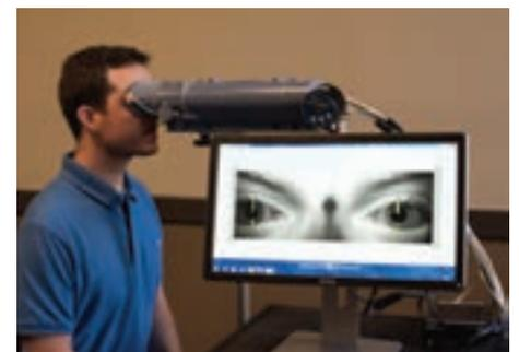
**A prototype of the Blink device tracks eyelid movement to indicate possible concussion.**
